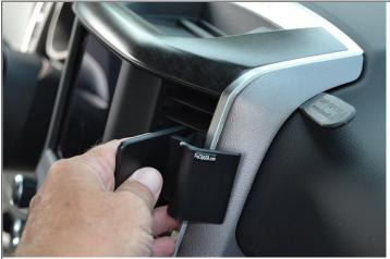
2. The adhesive tape cover must be removed. Place the ProClip in your hand so the ProClip label (sticker) is in an upright position on the upper right.
