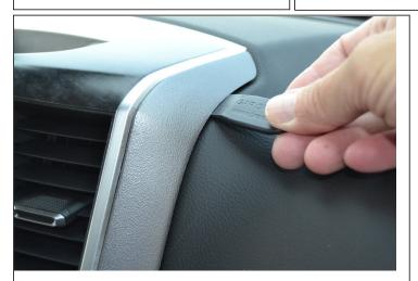
1. Clean the area where the ProClip will attach. Press the thin end of the enclosed gap opener into the gap between the upper center console frame and the padded dash top, to widen the gap.
