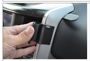
3. Push firmly forward on the right side of the ProClip face plate with your thumb so the angled edge flexes forward and hooks into the gap below gap opener.
